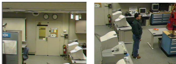
Figure 4: (a) The door and (b) the person whose height has been estimated from the PTZ camera calibrated using procedure described in this paper. The person is standing at point 6 shown at Figure 1. The points on the person and the door have been manually selected.
