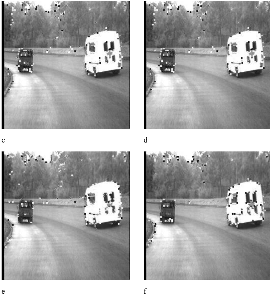
Figure 3.5: Potential corners for the ambulance sequence a), and corner maps obtained using: b) MIC algorithm; c) Harris corner detector; d) Modified Harris corner detector; e) Susan corner detector; and e) Wang and Brady algorithm.
