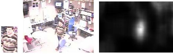
Figure 5: A template, an image and the histogram similarity function. Red areas correspond to high, while blue areas correspond to low similarity.
